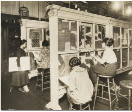
Students looking at textiles, ca. 1925. Textiles, which could not be handled, necessitated the invention of display cases with interior sliding panels. (Courtesy Cooper Hewitt, Smithsonian Design Museum)
